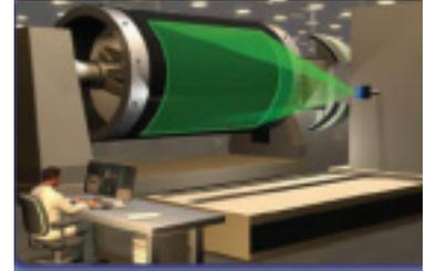
Remote inspection removes the inspector from the work envelope, enabling production and inspection to occur in parallel, rather than in series. The system adds material while inspection is occurring in a safer, more amenable location. Human inspection is also improved through image magnification and contrast enhancement. On-screen gauging applied to the image improves the quality of the documentation.
